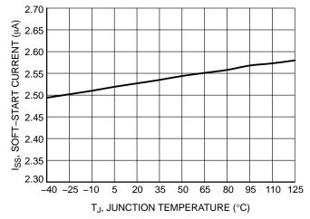
Figure 10. Soft-start Current vs. Temperature
