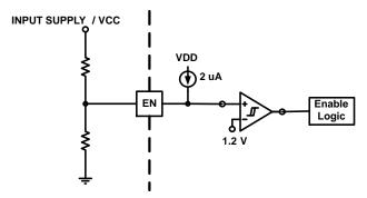
Figure 28. Enable Functional Block Diagram
