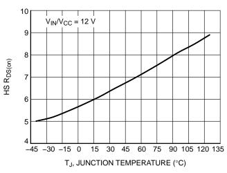
Figure 11. HS R<sub>DS(on)</sub> vs. Temperature
