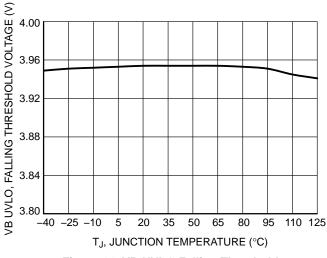
Figure 14. VB UVLO Falling Threshold vs. Junction Temperature
