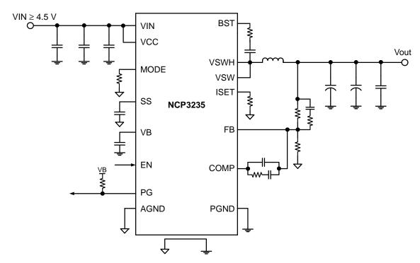
Figure 2. NCP3235 Typical Application Circuit Without External VCC
