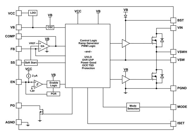
Figure 1. NCP3235 Block Diagram
