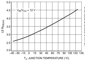
Figure 12. LS  $R_{DS(on)}$  vs. Temperature
