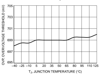
Figure 15. Output OVP vs. Junction Temperature
