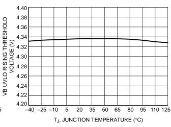
Figure 13. VB UVLO Rising Threshold vs.
