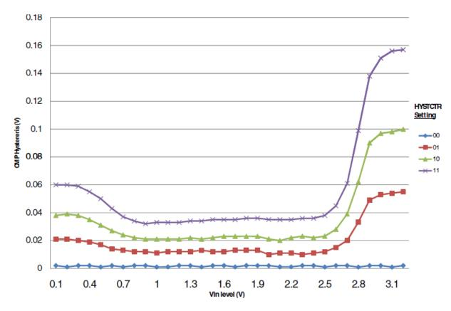
Figure 13. Typical hysteresis vs. Vin level (VDD=3.3 V, PMODE=1)
