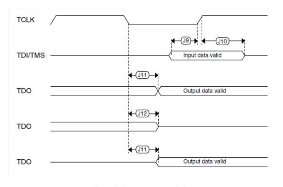
Figure 5. Test access port timing
