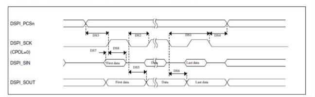
Figure 16. DSPI classic SPI timing — master mode
