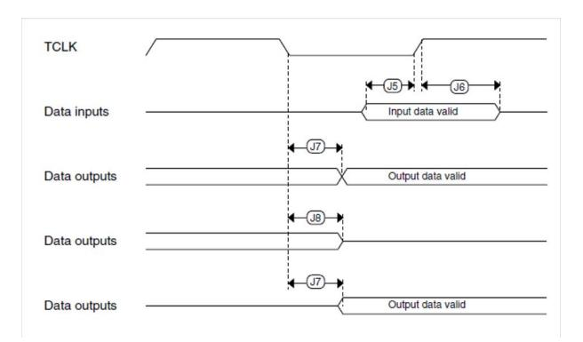
Figure 4. Boundary scan (JTAG) timing
