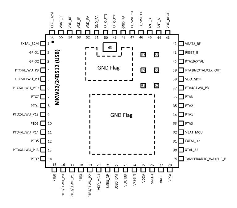
Figure 25. MKW22/24D512V (USB) Pin Assignment
