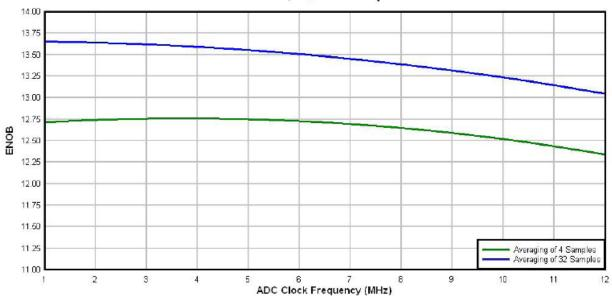
Figure 11. Typical ENOB vs. ADC\_CLK for 16-bit single-ended mode
