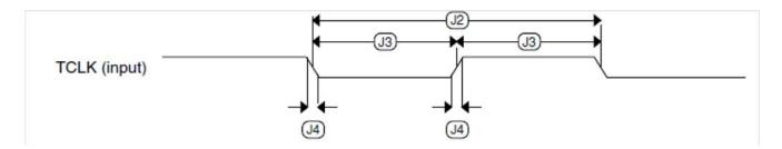
Figure 3. Test clock input timing
