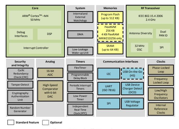
Figure 1. MKW2x simplified block diagram
