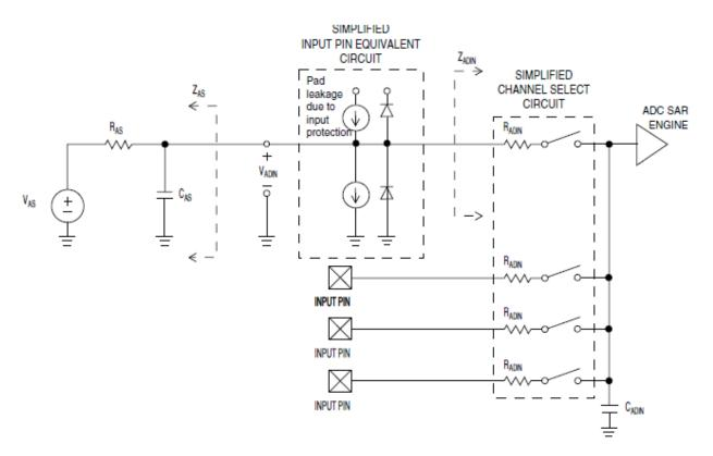
Figure 9. ADC input impedance equivalency diagram
