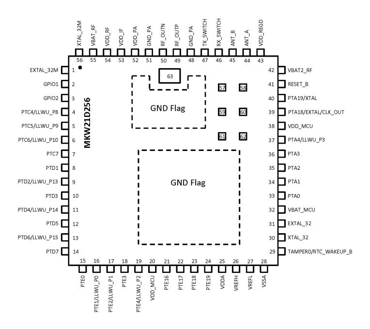
Figure 24. MKW21D256V Pin Assignment
