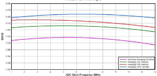
Figure 10. Typical ENOB vs. ADC\_CLK for 16-bit differential mode
