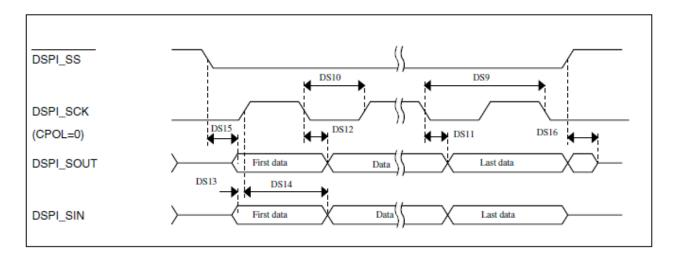
Figure 15. DSPI classic SPI timing — slave mode
