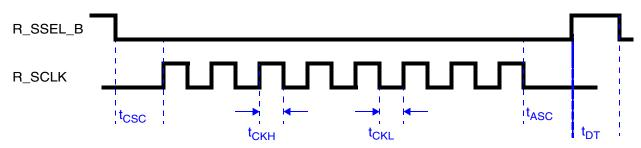
Figure 22. SPI timing: R\_SSEL\_B to R\_SCLK
