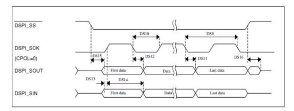
Figure 17. DSPI classic SPI timing — slave mode
