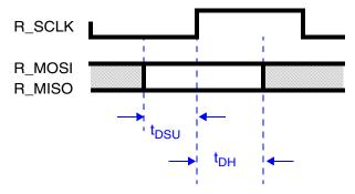
Figure 23. SPI timing: R\_SCLK to R\_MOSI and R\_MISO
