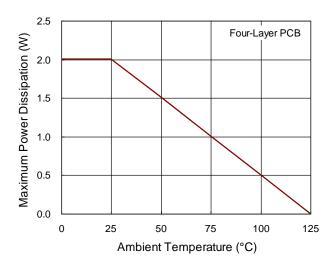
Figure 2. Derating Curve of Maximum Power
