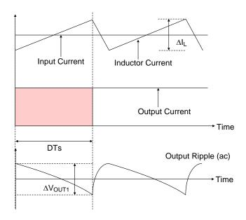
Figure 1. Output Ripple Voltage Without Contribution of **ESR**
