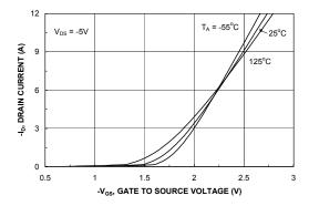
Figure 5. Transfer Characteristics.
